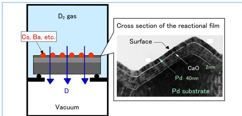
**Figure 1 Method of transmutation by D<sub>2</sub> gas permeation**
