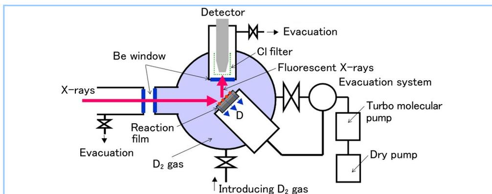
Figure 3 Experimental device used for in situ measurement in SPring-8
